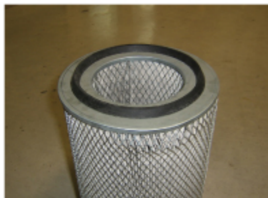
1.主滤芯已破损
