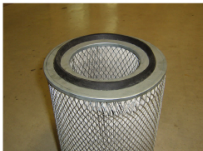
1.主滤芯已破损
