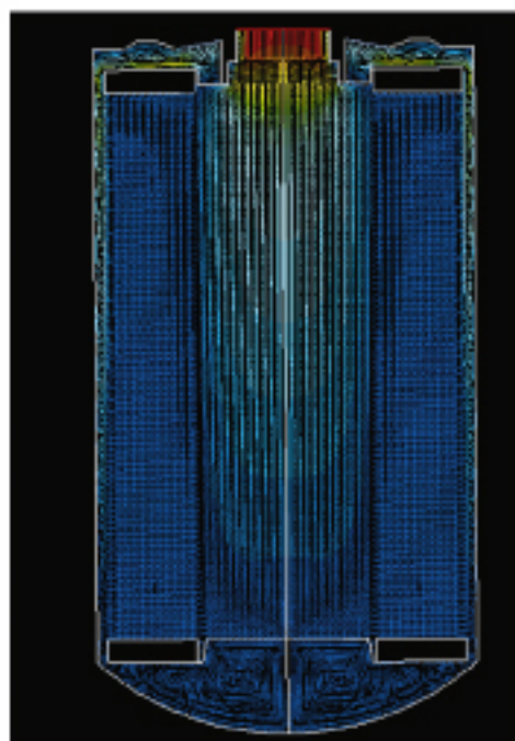
液体滤清器CFD流线图，显示流场中各点速度大小及方向 Flow path of liquid filter flow field, displaying vectors
